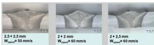
Fig. 9. LHW joints of DP 1000 steel sheets with filler material using LHW in keyhole mode at CLUPM.
