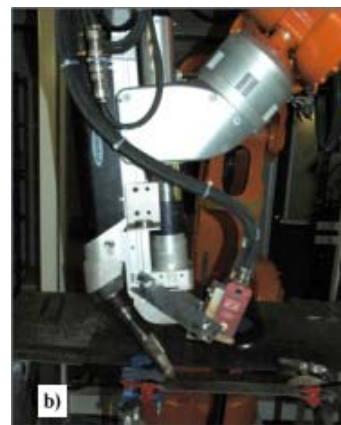
Fig. 6. ABB robot operating a Nd:YAG laser beam at CLUPM for: a. laser welding b. laser hybrid welding.
